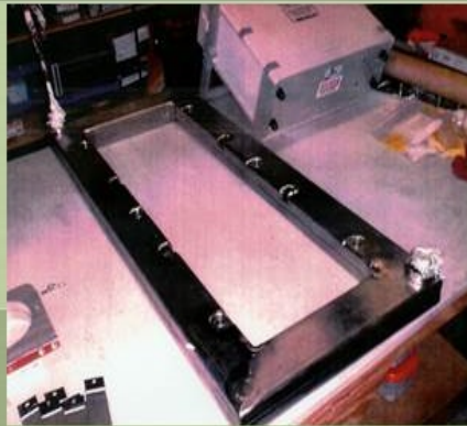
NbTi Superconducting Loop Enclosed in Stainless Steel Jacket that Contains Liquid Helium Coolant
