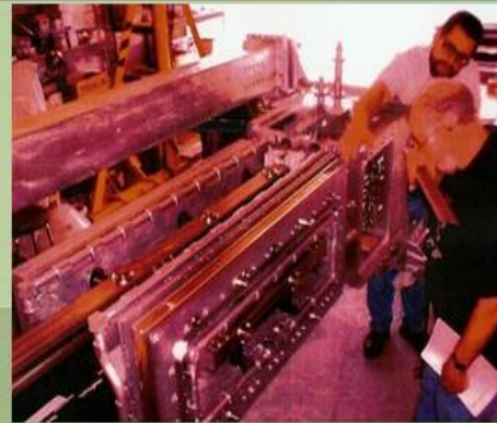
Assembly of Maglev 2000 Superconducting Quadrupole into Cryostat— Successfully Tested at Design Current of 600,000 Amps
