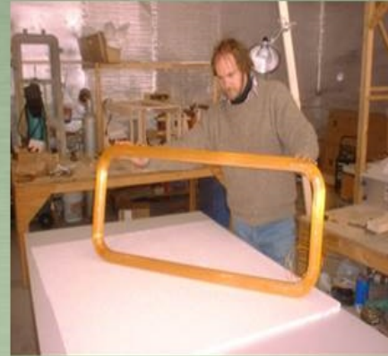
Assembly of Maglev 2000 Superconducting Quadrupole into Cryostat— Successfully Tested at Design Current of 600,000 Amps
