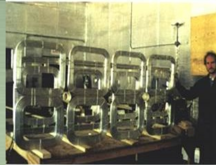
Completed Guideway Panel with Figure of 8 Dipole, and LSM Propulsion Loops
