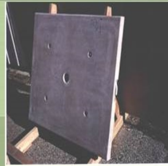
Polymer Concrete Panel with Enclosed Aluminum Loop Exposed for 2 years to Outdoor Environment with Multiple Freeze-Thaw Cycles
